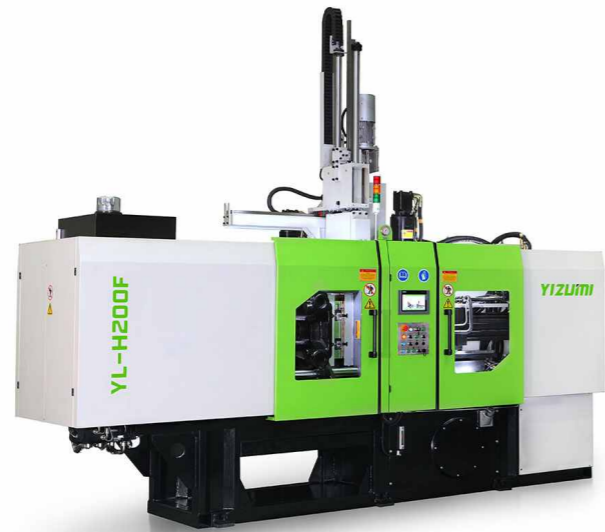
YL-H200F single cylinder (D3 clamping unit)
