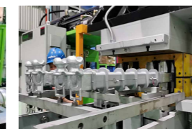
Part Name: 20kV Composite Crossarm Number of Cavities: 4
