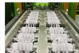
Part Name: 11 kV Arrester Number of Cavities: 16
