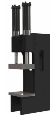
D4 Structure: C-frame 2-step downward closing; Features: Column free structure, 3-side operation accessible, double sliding plate or rotary table available to achieve double lower mold exchange; Downward closing structure, inserts will not move.
