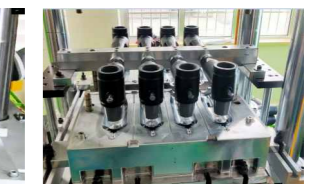
Part Name: 10kV T Joint Number of Cavities: 8
