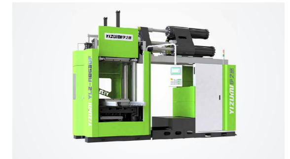
YL2-AB630F (Injection volume 10000cm 3 , injection pressure 1700bar)
