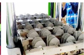
Part Name: 11 kV Composite Insulator Number of Cavities: 24
