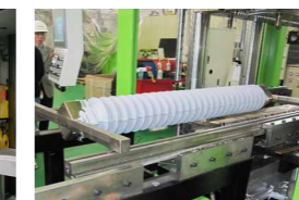
Part Name: 110kV Arrester Number of Cavities: 1
