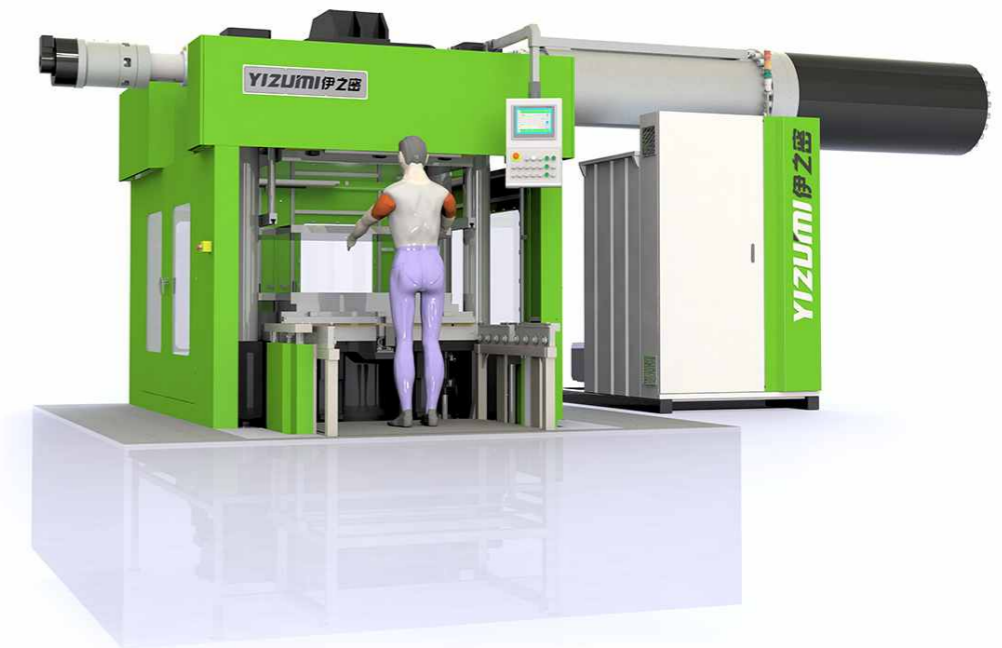
YL2-AB1200L ( Injection volume 40000cm 3 , injection pressure 1900bar )
